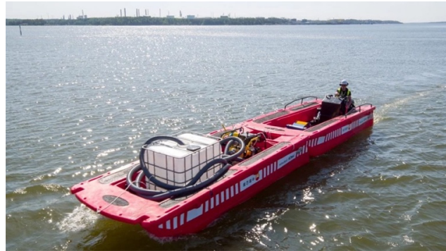
Figure 4 - Lamor Seahunter work platform: two units attached in tandem with an onboard oil storage tote.
